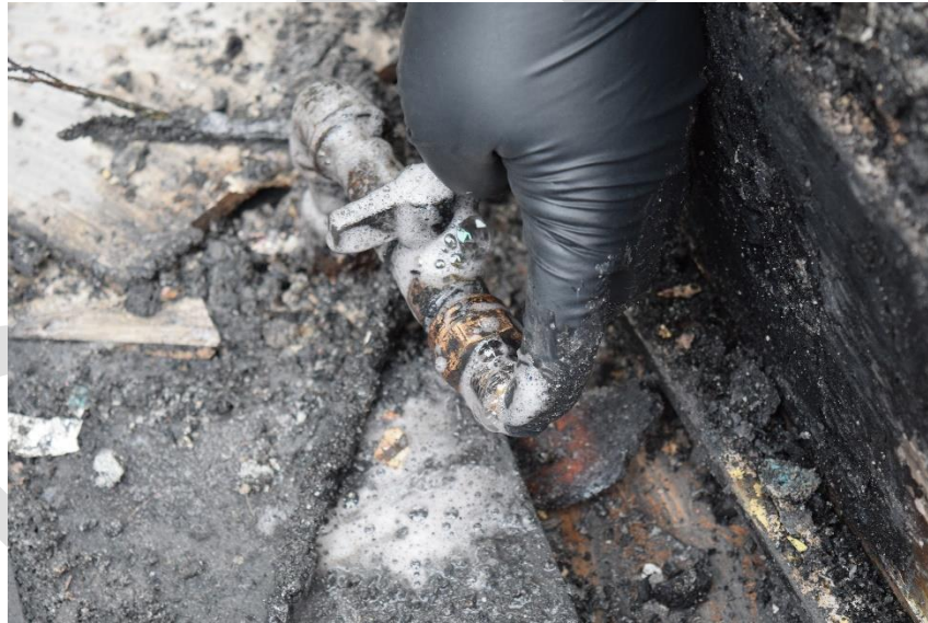
Figure 5 – Soap test on house piping showing bubbles forming near valve. Image provided by MVFD.
