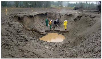
2003 rupture (with no ignition) of a natural gas transmission pipeline near Toledo, WA
